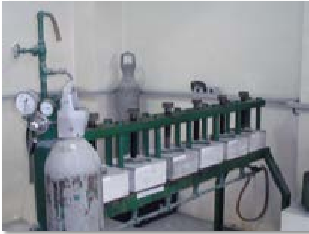
Penetration of water under pressure – NBR 10.787/94 (April 2007) Concrete: CII-E 32 at IPT (Technological Research Institute of São Paulo State), Brazil
