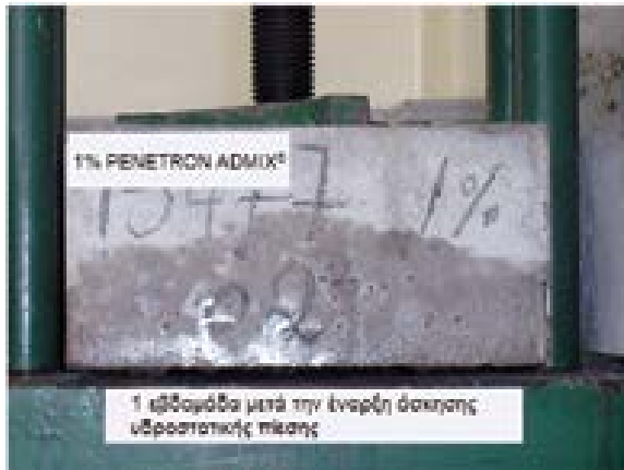
Penetration of water under pressure – NBR 10.787/94 (April 2007) Concrete: CPII-E 32
